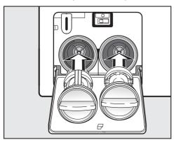
Replace the filters correctly (on the right and left) and tighten them.
