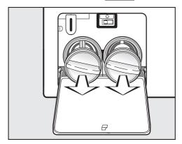
■ Remove the filters completely.
