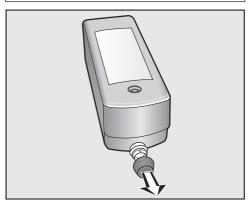
■ Remove the stoppers from the detergent cartridges.
