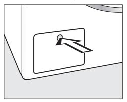
■ Press the drain pump access panel.
