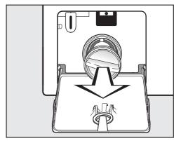
■ Remove the drain filter completely.
