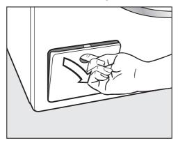
Open the drain pump access panel.
