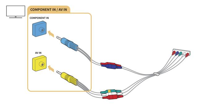
To use component equipment, connect both the component adapter (blue) and the AV adapter (yellow).
