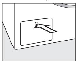
■ Press the drain pump access panel.
