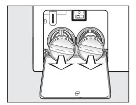
■ Remove the filters completely.
