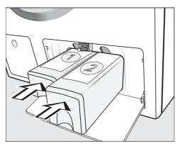
Push the UltraPhase 1 cartridge into compartment 1 and the UltraPhase 2 cartridge into compartment 2, until they lock into position.
