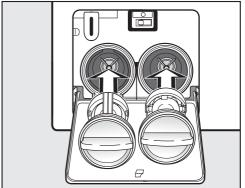
Replace the filters correctly (on the right and left) and tighten them securely.
