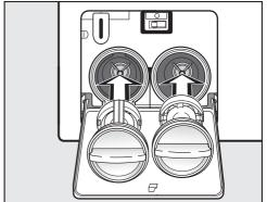
Replace the filters correctly (on the right and left) and tighten them securely.
