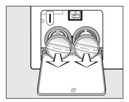
■ Remove the filters completely.
