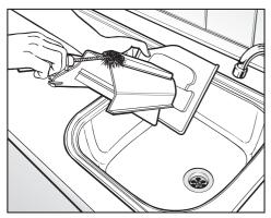
Clean the fabric softener channel using a brush and warm water.
