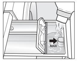
■ Add the fabric softener or liquid starch to the ⊗ compartment or insert the appropriate capsule. Do not exceed the maximum level mark.
