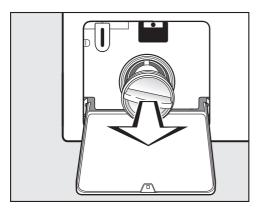
■ Remove the drain filter completely.
