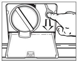
■ Pull the emergency release downwards. The door will open.
