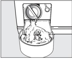
■ Slowly and carefully unscrew the drain filter to let the water out. Be careful not to release too much water at once. If the flow of water is too strong, some water can seep into the washing machine base and activate the water protection float switch. This will prevent the washing machine from functioning.
