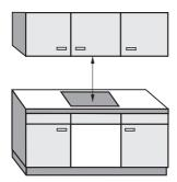
A minimum safety distance must be maintained between the cooktop and the rangehood above it. See the rangehood manufacturer's operating and installation instructions for details.
