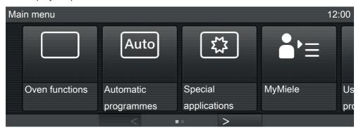
The menu path appears at the top left and shows you which menu or sub menu you are in. Options within a menu are separated by a vertical line. If there is not enough space to show the whole path, additional options are indicated by ... I. The time of day, alarm 1 and minute minder 1 are shown at the top right hand side of the display.
