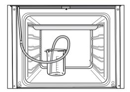
Place the container with the descaling solution on the floor of the oven.
