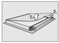
■ **Gently** lift the inner pane up and out of the plastic strip.
