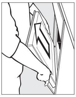
■ Hold the door securely at both sides, and lift it upwards off the retainers.
