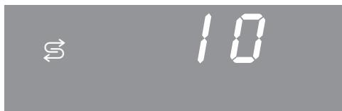
You can use the Moisture Plus
