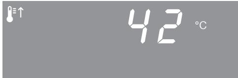
You can follow the temperature increasing. A buzzer will sound when the required oven temperature is first reached if this option is selected (see "Settings - P 2").
