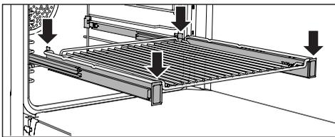
The maximum load for the FlexiClip telescopic runners is 15 kg.
