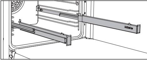
The FlexiClip telescopic runners can be attached to any shelf level.
