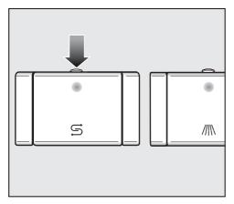
Press the button on the lid of the salt reservoir in the direction of the arrow.
