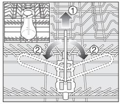
■ If the bottle holder is not needed, lift it up ① and fold the sides down ②, as illustrated.
