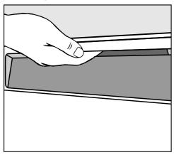
To open the door, reach under the door grip and pull.
