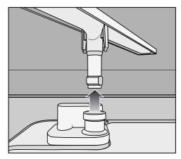
Pull the **lower** spray arm firmly upwards to remove it.
