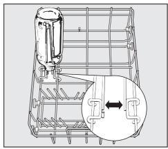
Place the bottle holder in the position shown in the bottom basket. If placed anywhere else, water will not be able to access the bottle properly, and cleaning results will be impaired.
