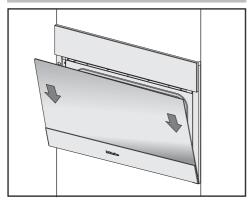
Hold the door securely at both sides and carefully fit it back onto the hinge guides. Risk of damage to the door.
