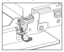
Release the locking clamps on the hinges by pushing them down. Turn them as far as they will go in an angled position. Danger of injury from the hinge guides for the door.
