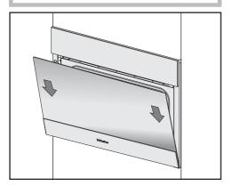
■ Hold the door securely at both sides and carefully fit it back onto the hinge guides.
