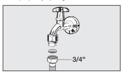
Connect the straight end of the stainless steel hose to the tap.
