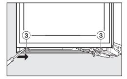
Using a flat-bladed screwdriver, slide the SoftClose mechanism towards the appliance side of the door.
