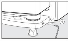
■ Undo grub screw ① with a full turn of the Allen key supplied.
