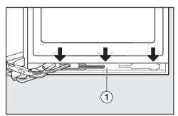
■ Prise open panel ① from the SoftClose mechanism: Insert a flat-bladed screwdriver into the gap from below and ease off the panel bit by bit.
