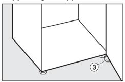
■ The foot ③ should **definitely** be unscrewed until it rests on the floor. Then turn it a further 90°.
