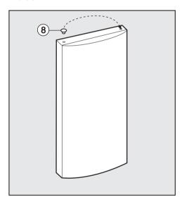
■ Remove cap <sup>®</sup> from the bearing bush in the door and refit on the opposite side.
