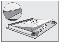
■ Refit the bottom of the two middle panes. The more angled corner must be located at the bottom left.
