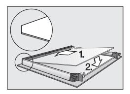
■ Refit the top of the two middle panes. The more angled corner must be located at the top left.
