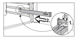
■ Hook the FlexiClip telescopic runner onto the bottom rail of a shelf level at the front (1.) and push it along the rail into the oven interior (2.).
