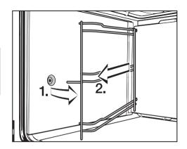
■ Pull the runners out of the holder (1) at the front of the oven and then pull them out of the oven (2).
