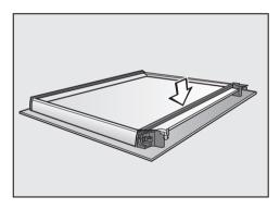
■ Refit the fibreglass seal.
