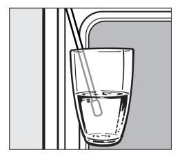
Immerse the end of the water intake pipe in the container with tap water.
