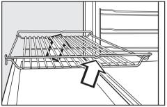
Always place the rack in the shelf runners with the non-tip safety notches towards the back.
