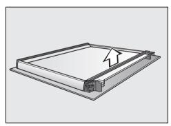
■ Remove the fibreglass seal.
