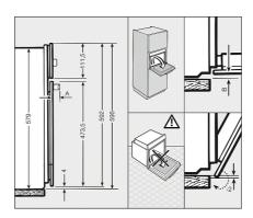
Detailed installation drawing H 6000,H 5000, H 4000, E/B, EP/BP, 76 litres, (Installation drawing)
