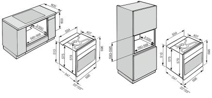
H 5000 E/B; H 47xx E/B, H 48xx E/B; H 6000 E/B; H 2000 E/B - 60 cm (Installation drawing)
