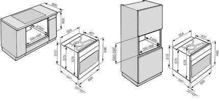
H 5000 E/B; H 47xx E/B, H 48xx E/B; H 6000 E/B; H 2000 E/B - 60 cm (Installation drawing)
