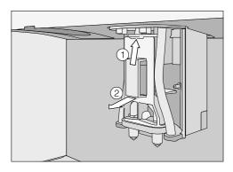
■ Press the catch ① upwards, grasp the dispensing unit by the handle and pull this forwards and off ②.
