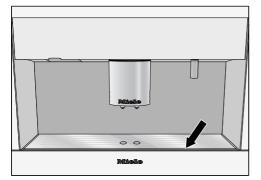
■ Refit the cover in the drip tray. Make sure the drip tray cover sits flush at the front.
