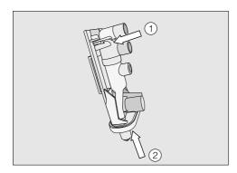
■ Reassemble the spout unit in the reverse order. Make sure the top connection piece ① engages with a click. Firmly push the spout jets ② onto the dispensing unit.
