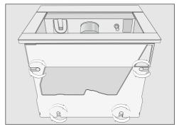
■ Using the large allen key, unscrew all four feet out by about 2 mm.
