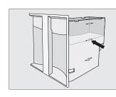
Fill the water container with lukewarm water up to the level marker ///\ and add 1 sachet of the Original Miele cleaning agent for milk pipework. Push the water container back into the machine.
