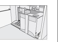
■ Fill the water container with fresh, cold tap water up to the "max."
