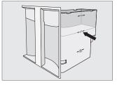
■ Fill the water container to the marker \$\mathcal{S}\$ with lukewarm water and drop two Miele descaling tablets in the water. Push the water container back into the appliance.
