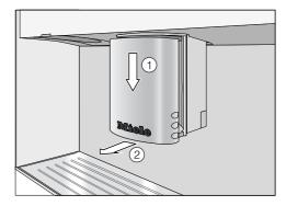
■ Push the central spout right down ① and remove the cover by pulling it off towards you ②.
