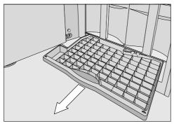
Open the machine door and carefully remove the drip tray from the machine.
