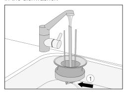
Rinse the milk pipework in the lid under running water.
