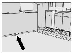
Remove the drip catcher and clean it in the dishwasher or by hand using warm water and a little washing-up liquid applied with a soft cloth.
