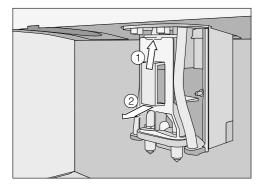
■ Press the catch ① upwards, grasp the dispensing unit by the handle and pull this forwards and off ②.
