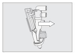
■ Hold the unit at the sides and pull it forwards to release it.
