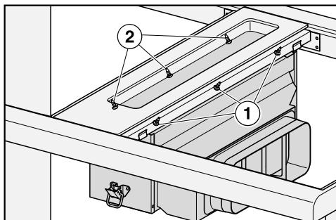
■ Fasten the casing from the inside with the screws ① on the right and left ② sides (3 in each case).
