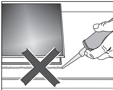
The SmartLine appliance and worktop may be damaged if the appliance needs to be removed after it has been sealed with a sealant. Do not use any sealant between the SmartLine appliance and the worktop. The sealing strip under the edge of the top part of the appliance provides a sufficient seal for the worktop.
