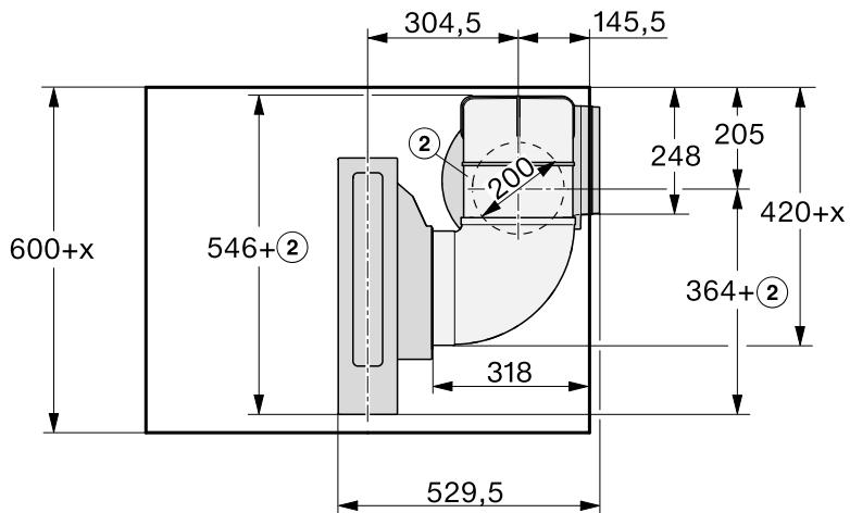
If you want to install the air duct to the left of the downdraft extractor, the worktop must be at least 665 mm deep.
