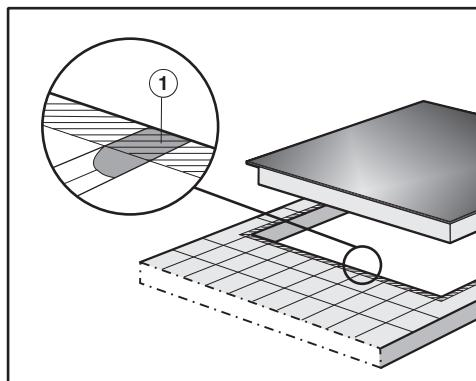
Grout lines ① and the hatched area underneath the SmartLine appliance frame must be smooth and even. If they are not, the SmartLine appliance will not sit flush with the worktop and the sealing strip underneath the top part of the appliance will not provide a good seal between the appliance and the worktop.
