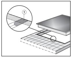
Grout lines ① and the hatched area underneath the CombiSet frame must be smooth and even. If they are not the CombiSet will not sit flush with the worktop and the sealing strip underneath the top part of the appliance will not provide a good seal between the appliance and the worktop.
