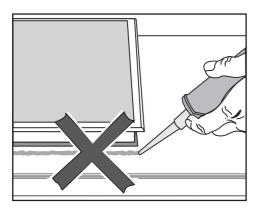
Do not use sealant between the CombiSet and the worktop. This could result in damage to the CombiSet or the worktop if the CombiSet ever needs to be removed for servicing.
