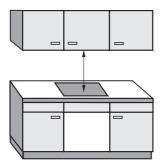
A minimum safety distance must be maintained between the CombiSet and the rangehood above it. See the rangehood manufacturer's operating and installation instructions for details.
