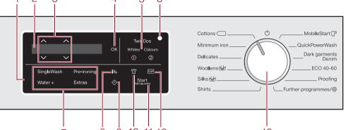
Control panel The control panel consists of a display and various sensor controls.
