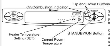
Setting or adjusting the room temperature can only be performed while the appliance is in operation, press the "STANDBY/ON" button once to turn the heater on.
