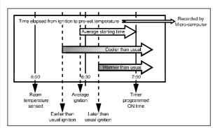
This function is called Pre-heat since it ensures the room reaches the desired temperature by the time the Timer programs ON time. The room temperature is sensed one hour before reaching Timers programmed ON time.
