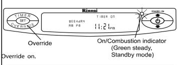
This function is used to manually override the current operation of the heater. For example: if the heater is between the finishing and starting times of a timer program and the Override button is selected, then the heater will begin to operate and heat the room.
