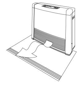
During peak operating periods the filters should be cleaned weekly, however if the "FILTER" warning indicator flashes in the control panel display, turn off the appliance immediately and clean filters before further use.
