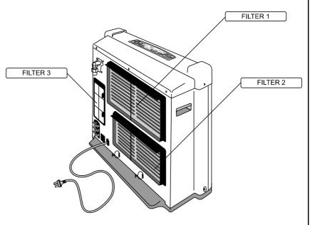
Replace filters by carefully repositioning the location tabs and fasten in place with the retaining screw.
