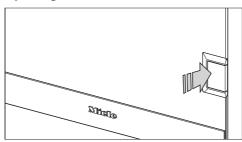
■ Open the door by pressing on the left hand side of the door release.
