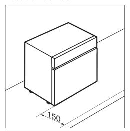
▶ The minimum safety distance between the front of the appliance door and the edge of the worktop is 150 mm.
