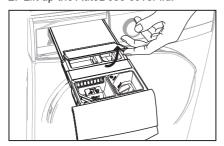
3. Gently pour only liquid detergent in the AutoDose detergent tank 🔊. Fill up to the maximum indicated level MAX.
