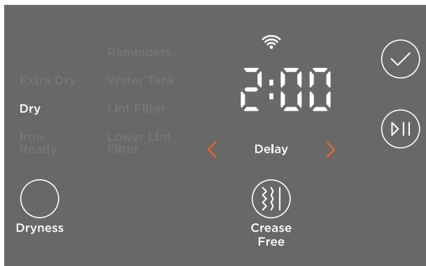
1. After setting the drying cycle, press **DELAY**, then use the arrows < or > to set your preferred delay duration.
