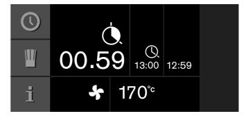
The appliance switches off after the cooking time has elapsed. The symbol flashes and a signal sounds. The signal stops when you touch the symbol, open the appliance door, or switch the function selector to 0.
