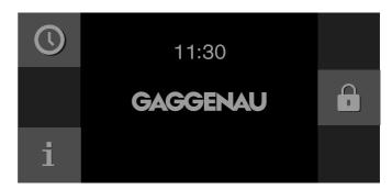
The child lock is activated. The standby screen appears. The ⊕ symbol is shown at the top of the display.
