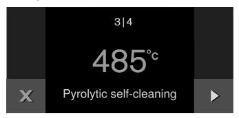
A signal sounds after 3 hours. A message appears in the display. Once the appliance has cooled down, wipe the remaining ash out of the interior with a moist cloth.
