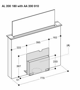
**A:** Access to the complete cover must be ensured even after installation
