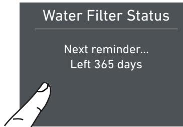
**E)** Here are indicated the remaining days before the due date for the substitution of the filter.
