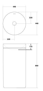
$Dimensions \ are \ shown \ in \ millimetres. \ Due \ to \ the \ handcrafted \ nature \ of \ Omvivo \ products \ measurements \ are \ subject \ to \ a +/- \ 5mm \ manufacturing \ tolerance.$
