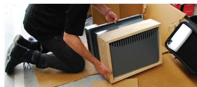
21 Note the four pre-drilled bolt holes on the interior of wall panel **11** – two above the conditioner cutout void and two below.
