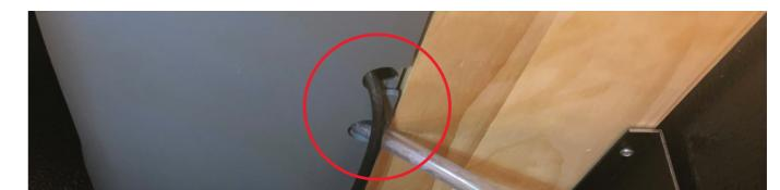
33 Lift the conditioner/frame assembly into position and attach it to wall panel **11** by carefully re-inserting the two **C5** bolts (including the wide washers this time) through the metal brackets (see warning after step 22 above).
