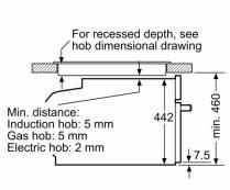
measurements in mm
