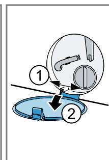
5. Slide a suitable receptacle under the opening for draining the detergent solution.
