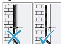
Do not trap the power cord or the hoses between the wall and the appliance.
