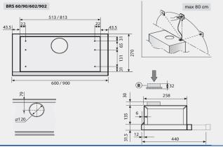
Method of Installation: Built into overhead cupboards
