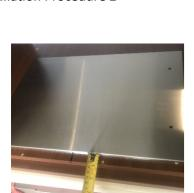
Sit the Base (part 3) on the melamine base with the centre notch at the front. Place it in 20mm from the front edge. Align the centre notch and the centre line marked to locate the base. Ensure the base front edge is parallel with the front.
