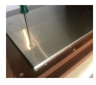
Screw the Base (part 3) to the melamine base panel using 2 x 6 gauge screws via two screw holes in the front corners. Do not screw too tight.
