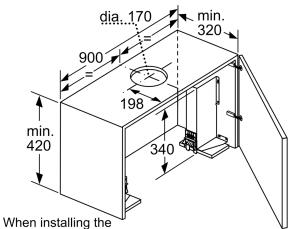
90 cm telescopic hood in a 90 cm wide wall-hanging cupboard, the mounting kit is required. The two mounting brackets are screwed onto the right and left of the kitchen unit. Installation in accordance with template.
