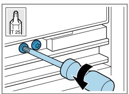
3. Adjust the door and tighten both screws.
