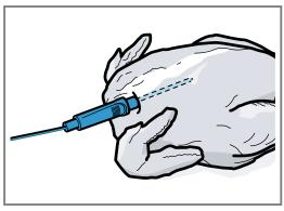
2. Depending on its composition, insert the core temperature probe into the poultry crossways or lengthwavs.
