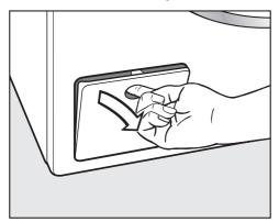
■ Open the drain pump access panel.
