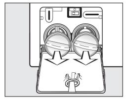
■ Remove the drain filters completely.
