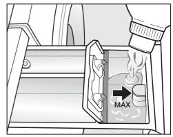
■ Add fabric conditioner or liquid starch to the % compartment. **Do not exceed the maximum level mark**.
