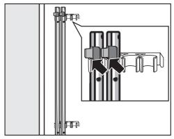
Secure the transit bars to the back of the washing machine. Make sure that the top catch is located above the holder.
