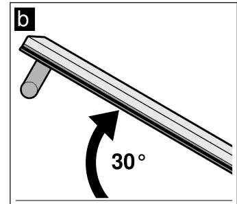
4. Lift the oven door slightly and pull it out.
