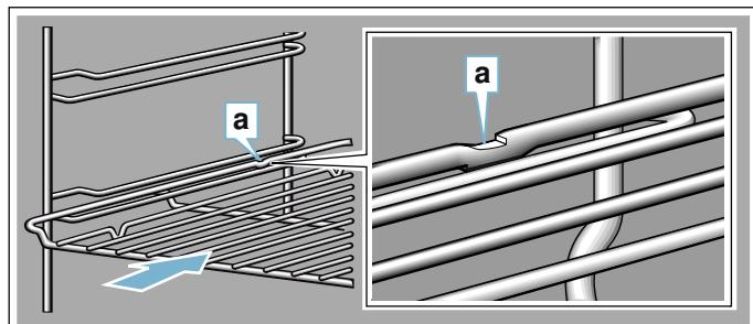
When inserting baking trays, ensure that the lug **a** is at the rear and is facing downwards. The sloping edge of the accessory **b** must be facing towards the appliance door.
