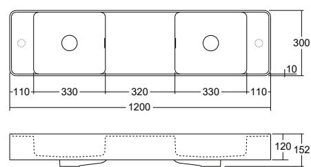
Dimensions are shown in millimetres. Due to the handcrafted nature of Omvivo products measurements are subject to a +/- 5mm manufacturing tolerance.
