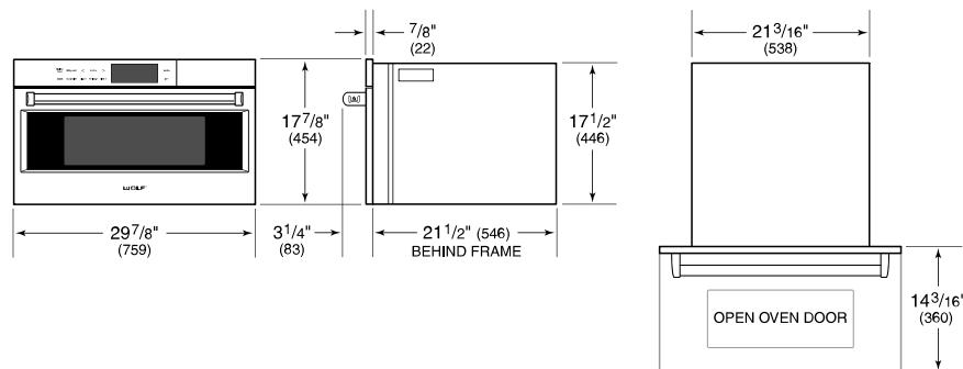
**NOTE:** Dimensions in parenthesis are in millimeters unless otherwise specified
