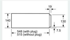
Compact ovens with an appliance height of 455 mm can be installed above a warming drawer.
