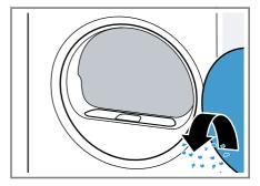
3. Remove the two-part fluff filter.
