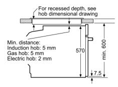
measurements in mm
