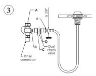
Ensure the black rubber washers are situated inside positions A, B, C, F and E on the rinse connector, including the double check non-return valve as shown in the diagram.
