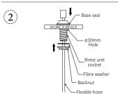
Secure the rinse unit socket in a suitable position using a tap wrench of a 36 AF spanner.
