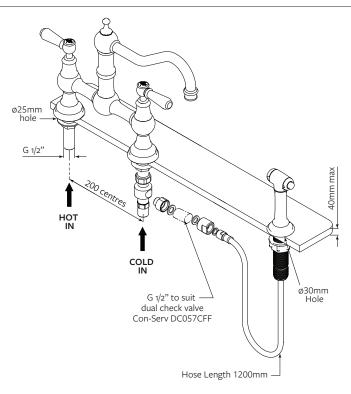
**Please Note:** This model does not suit incoming water pressure below 100kPa or higher than 500kPa. The spray rinse model requires a minimum inlet pressure of 100kPa to successfully divert the water flow from the main tap to the spray rinse. The stop cocks provided with this tap contain gauze filters. Please ensure your plumber is advised of the minimum and maximum water pressure, and to install the stop cocks as failure to do so voids the tap warranty.
